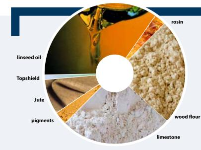
Forbo Marmoleum is created out of 97% natural raw materials, that are rapidly renewable, such as linseed, rosin, jute and wood flour, or available in abundance, like limestone. Forbo Marmoleum has the lowest LCA in the resilient flooring category, making it the most sustainable choice when it comes to choosing a floor.
