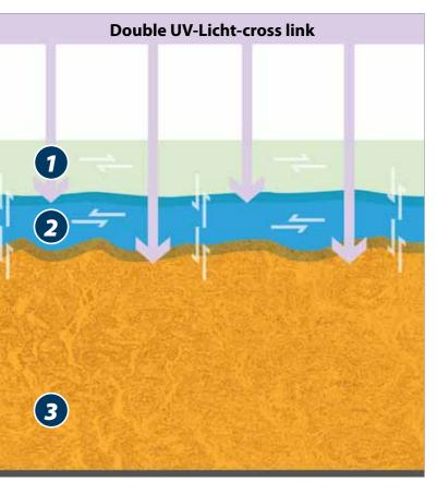
When developed in 2005 Forbo introduced Topshield with its characteristic double layer finish technology. The first layer acts as a primer that is flexible and elastic. The primer is UV cured creating a strong bond with the linoleum surface. The second layer is a tough surface finish that is dirt repellent and resistant to scratches and staining. With Topshield2 the formulation of both finish layers has been improved and this time also the topfinish layer is UV cured for even higher performance.
